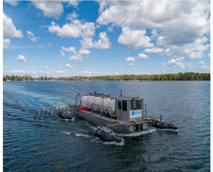
HAB Aquatic Solutions barge conducting the alum treatment
